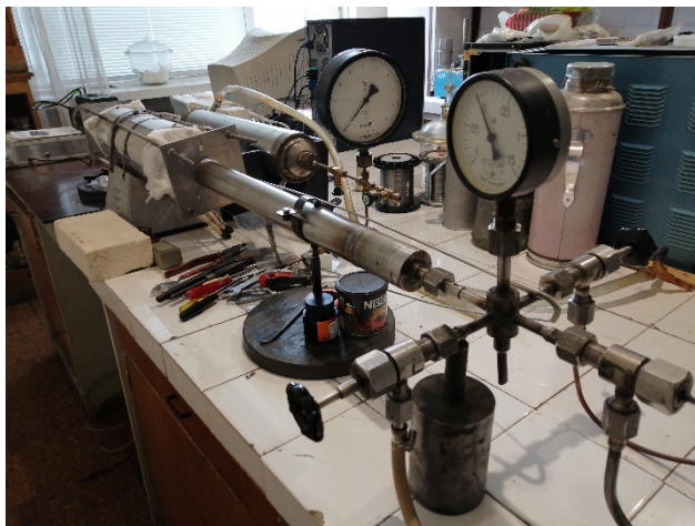
Fig. 3 General view of a laboratory chamber for hydrogenation
