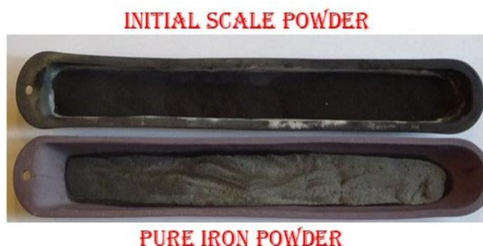
**Fig. 12. Image of initial scale powder before (dark colour) and after reduction – pure iron (light gray colour)**
