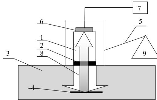
**Fig. 2. Probe PLU-6P-02 in working conditions. 1 - acoustic waveguide, 2 - Optical acoustic generator, 3 - sample, 4 - imperfection, 5 - optical cable, 6 - piezoelectric transducer, 7 - data acquisition and processing system (PC), 8 - ultrasonic pulse, 9 - laser.**
