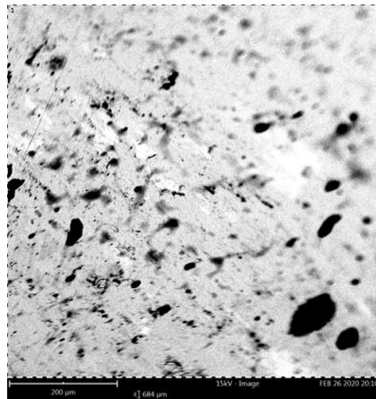
Fig.4 Image of a composite material based on iron powder with a Phenom ProX electron microscope.
