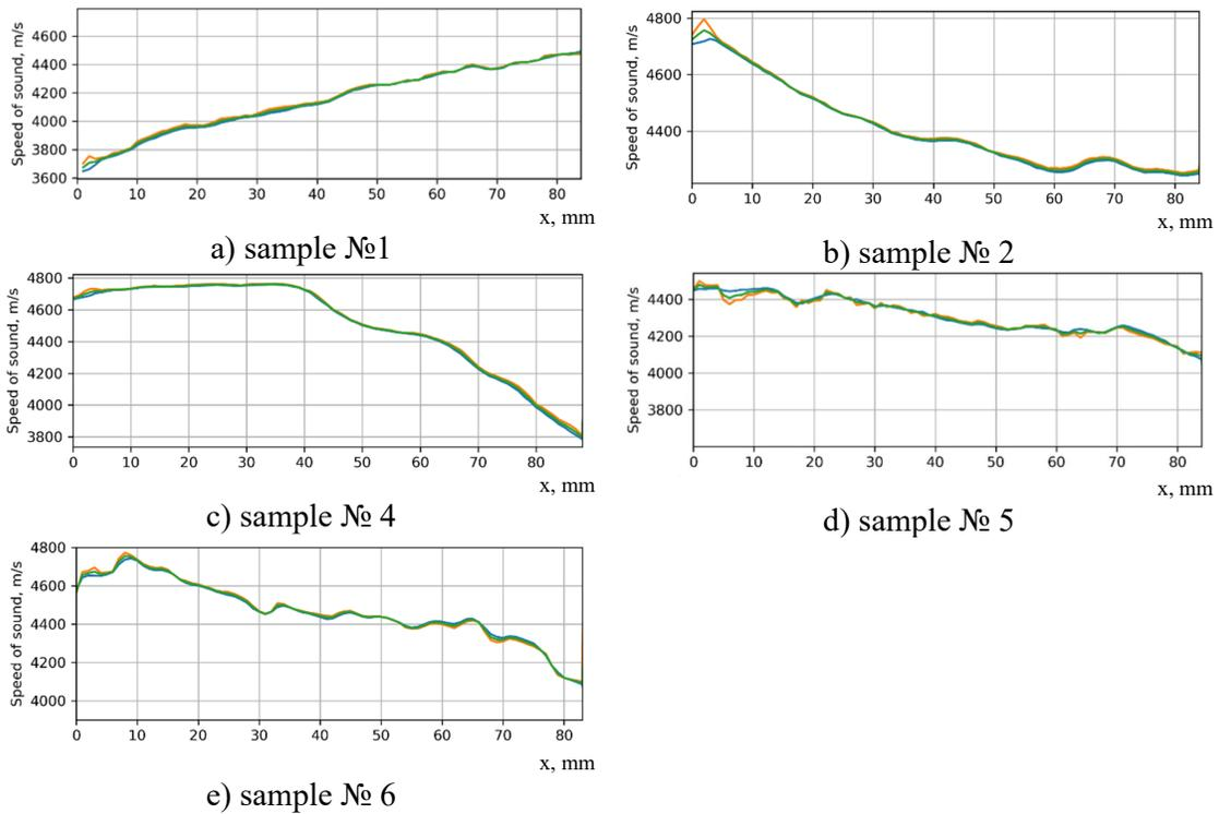
**Fig.6 Longitudinal wave propagation velocities distribution along the length of the specimens.**
