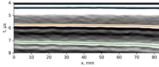
**Fig.5 Typical B-image from scanning with the laser ultrasound system of a composite material based on iron powder.**
