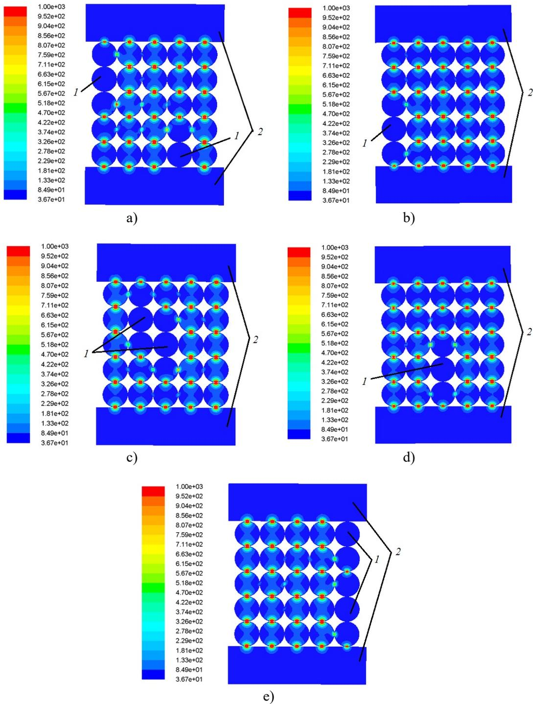
1 – PTFE particle, copper – other particles; 2 – electrodes
