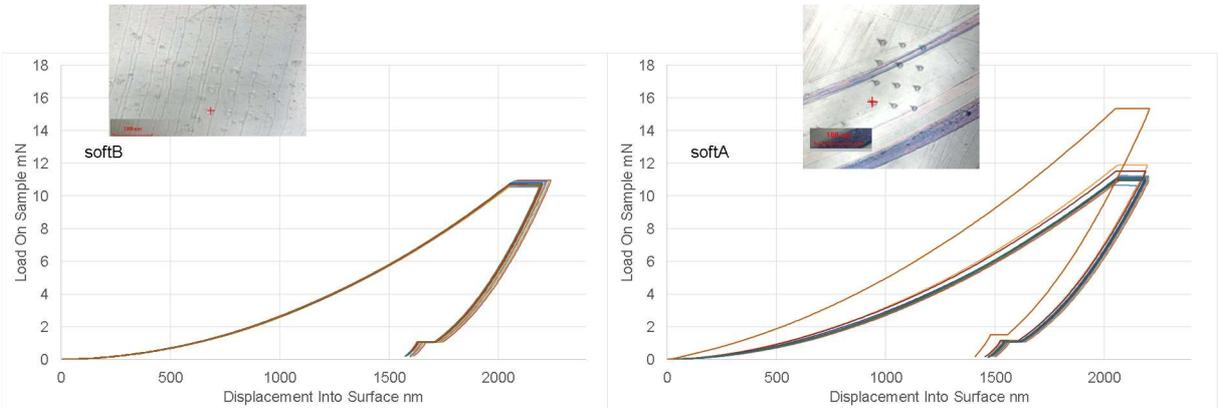
Fig. 4. Load displacement curves obtained via nanoindentation for PETG sample sheet of  $0.5 \text{ mm}$  thickness
