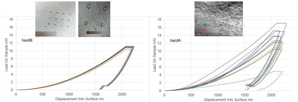
**Fig. 5. Load displacement curves obtained via nanoindentation for PETG sample sheet of 0.75 mm thickness**
