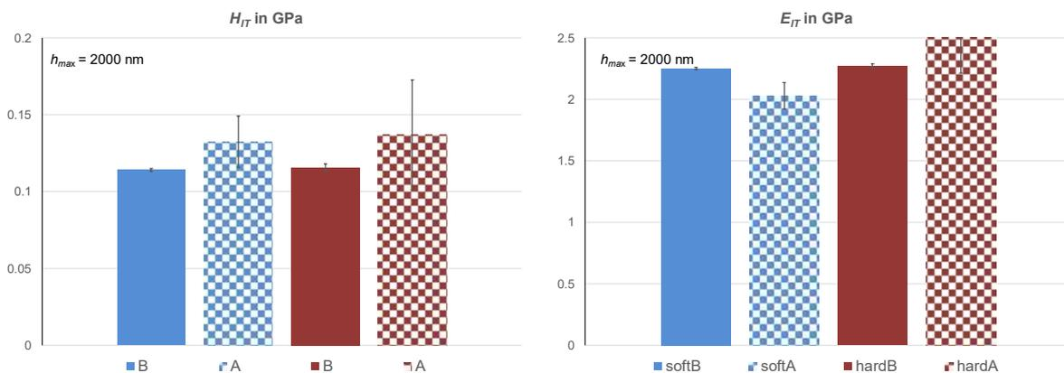
**Fig. 6. Nanoindentation hardness and elastic modulus of PETG before (denoted as B) and after (denoted as A) thermoforming**
