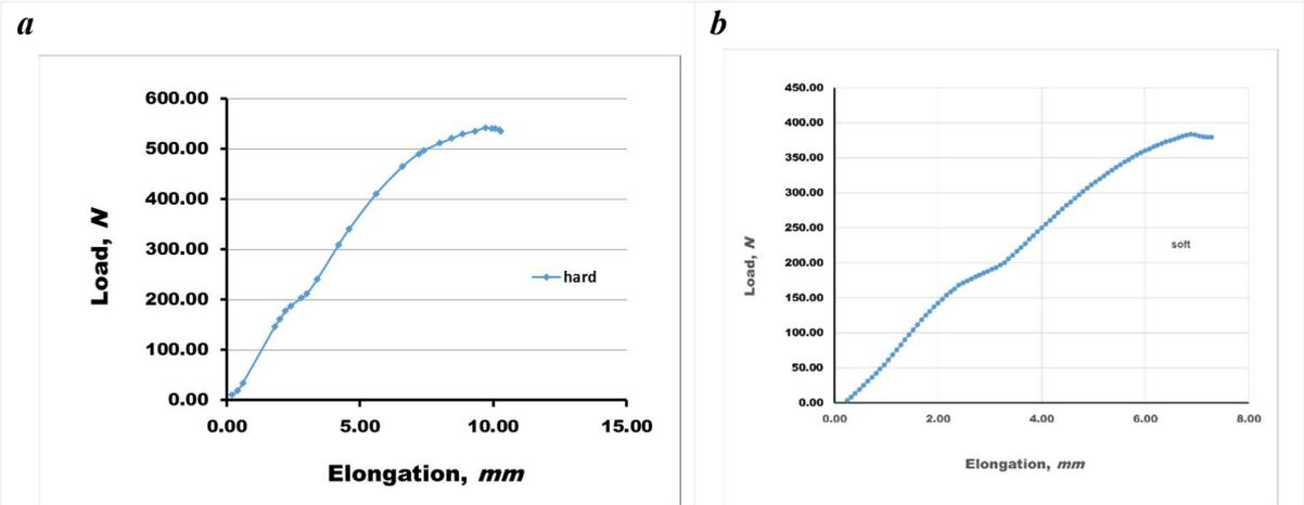
Fig. 3. Quasi-static tensile curves of dental PETG sheets of  $0.75 \text{ mm}$  (a) and of  $0.5 \text{ mm}$  (b) thickness values.
