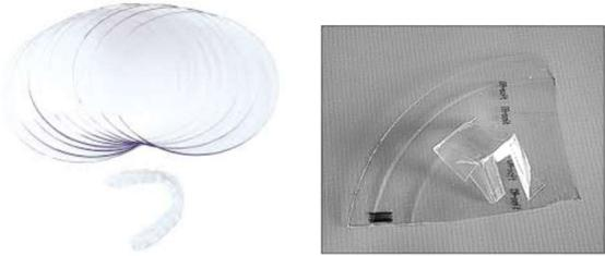
Fig. 2. PETG material and thermoformed sample
