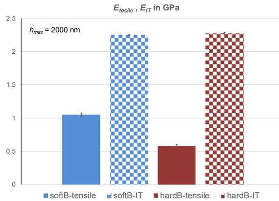
**Fig.7. Comparing the tensile test results vs. nanoindentation (IT)**
