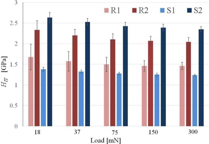
**Fig. 3. Indentation hardness vs. applied load onto the reference samples R-1 and R-2 and the space samples S-1 and S-2**
