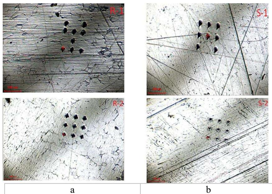
**Fig. 1. Imprints left by the Berkovich pyramid after nanoindentation onto the reference samples R-1 and R-2 (a), the space samples S-1 and S-2 (b)**
