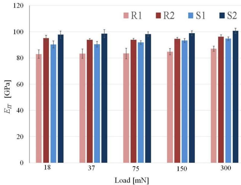
**Fig. 4. Indentation modulus vs. applied load onto the reference samples R-1 and R-2 and the space samples S-1 and S-2**
