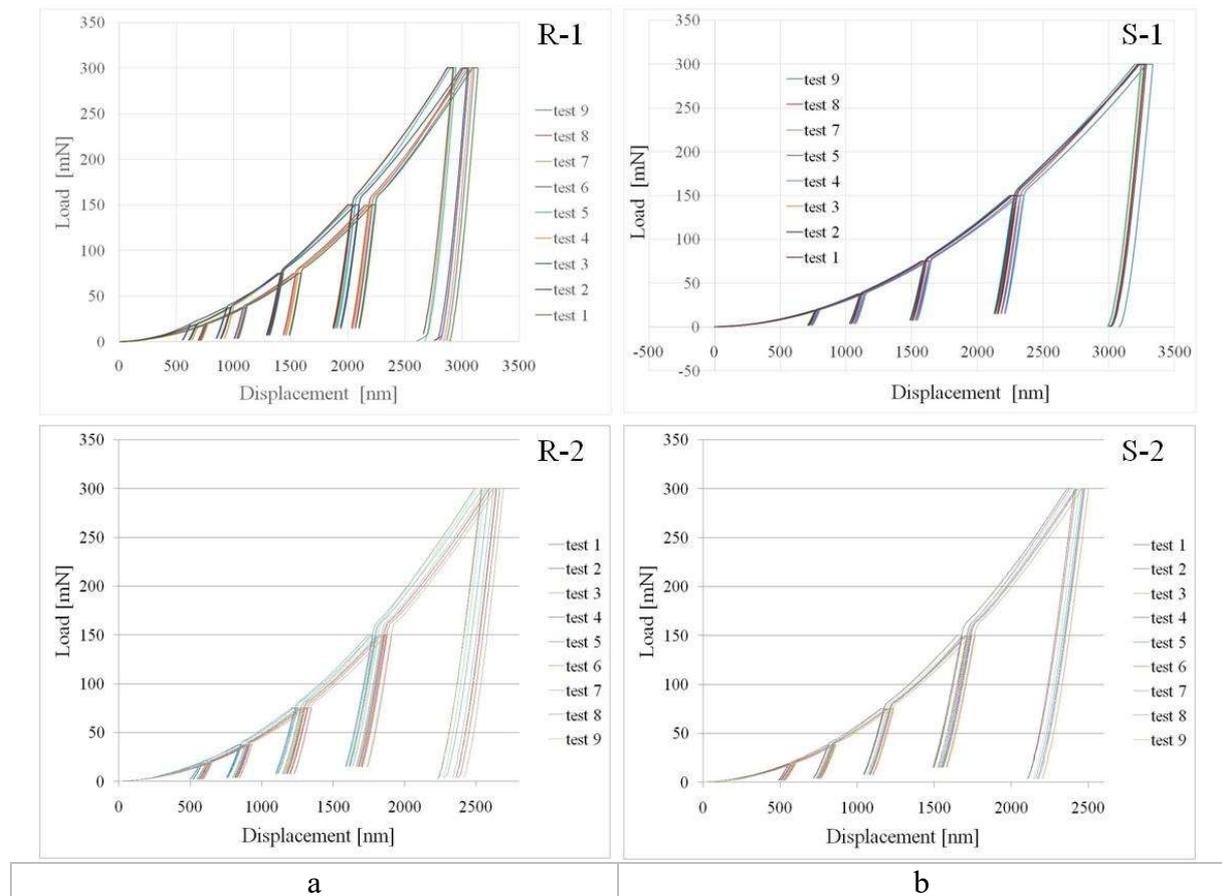
**Fig. 2 Indentation load-displacement curves for the reference samples R-1 and R-2 (a), the space samples S-1 and S-2 (b)**
