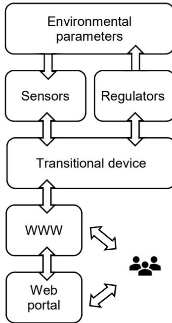
Fig. 1. Main scheme of the surveillance system of environmental parameters
