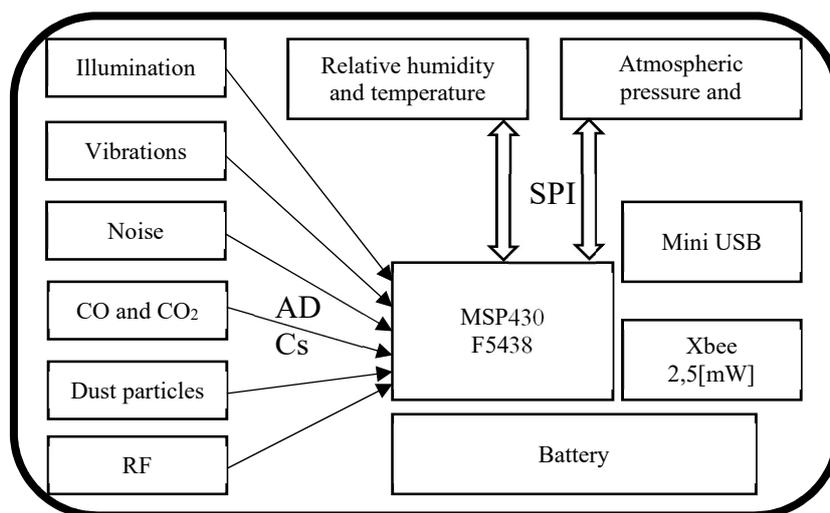
Fig. 2. Main scheme of the multisensor for monitoring and control
