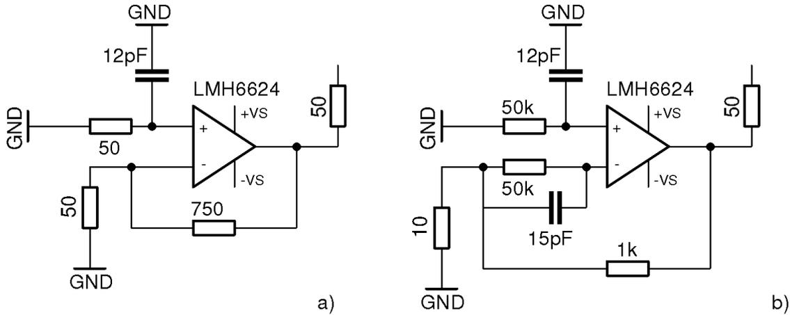
**Fig. 1 Preamplifiers' circuits**
