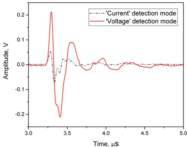
Fig.2. Signals detected by transducer with preamplifiers operating in voltage and current detection modes
