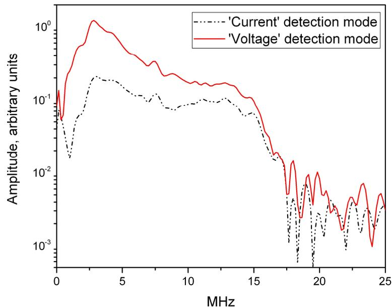
**Fig. 3. Spectra of the signals detected by transducer with preamplifiers operating in 'voltage' and 'current' detection modes.**
