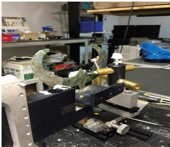
**Fig. 8. Crescent shaped application in X-ray diffractometer chamber
