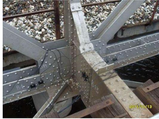
**Fig. 3.39 and 3.40. Moments of NDT with AE steel railway bridge at km 135+040 before the Stamboliyski station (left) and at km 154+004 in Plovdiv. (right)**
