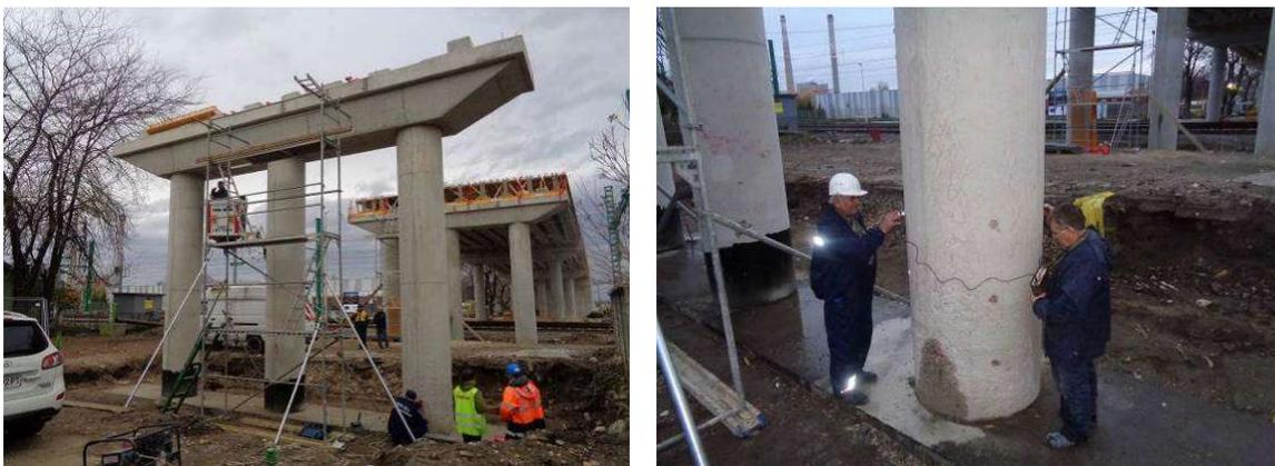
**Fig. 3.51 and 3.52 Moments from the ultrasonic studies of the homogeneity and the strength-deformation characteristics of the concrete in R/C columns of Road overpass Stamboliyski (2017)**
