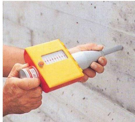
**Fig. 3.5 and 3.6. NDT reinforced concrete elements with "Schmidt" hammer type N (left) and type NR (right)**
