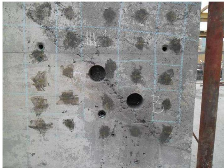
**Fig. 3.55 and 3.56. Moments of conducting ultrasonic examinations for the qualification of the R/C walls in a newly built Sugar products factory in Sofia (2014)**
