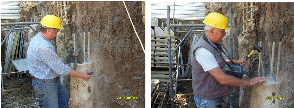
Fig. 3.37 and 3.38. Moments conducted by ultrasonic testing's: the velocity in concrete (left) and the integrity of piles (right) for strengthening the total excavation of the residential building in Sofia
