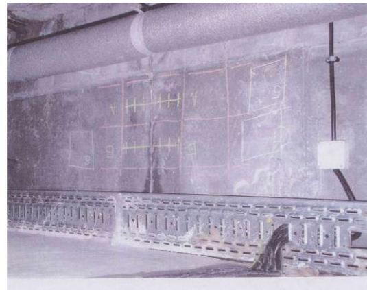
Fig. 3.17, 3.18. Fragment of the test zone with cracks and closer look (right) with the labeled bases to measure their depth by ultrasonic
