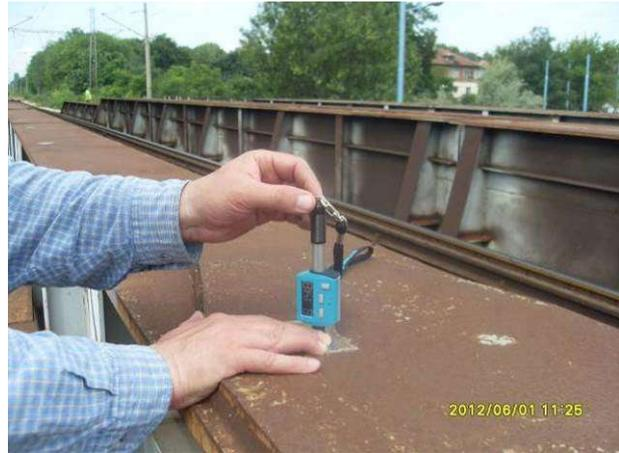
**Fig. 3.27 and 3.28 Remote Diagnostics of Slab Bridge Bearings (Left) and NDT of Steel Railway Bridge in Plovdiv (right) with EQUOTIP electronic hardness tester of Proceq**
