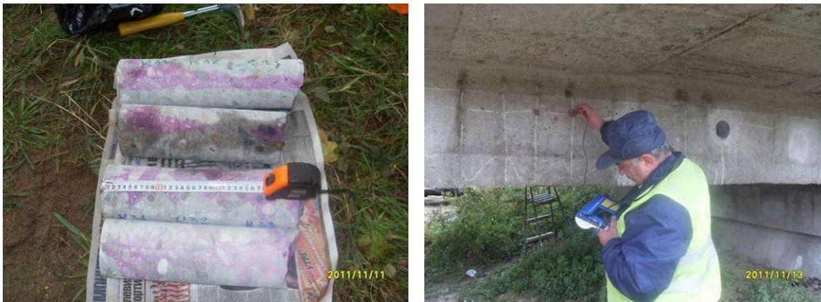
**Fig. 3.25 and 3.26** Determination of the depth of carbonation of concrete by a "colorimetric" method with a 5% solution of phenolphthalein in alcohol (left) and the potential for corrosion of the reinforcement with CANIN+
