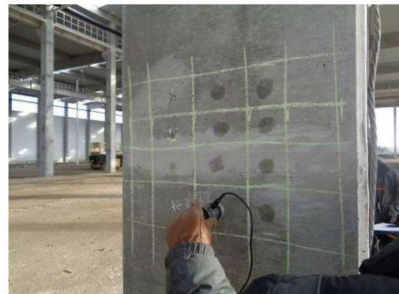
**Fig. 3.57 and 3.58 Moments of conducted ultrasonic examinations for qualified R/C columns in a newly built plastic craft factory in Shumen (2017)**
