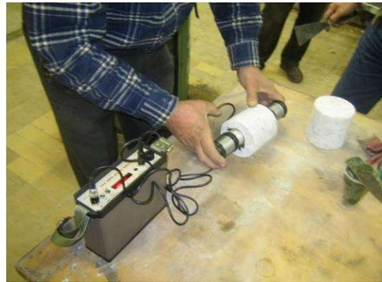
**Fig. 3.53 and 3.54 Moments of ultrasonic examination of cut concrete samples**
