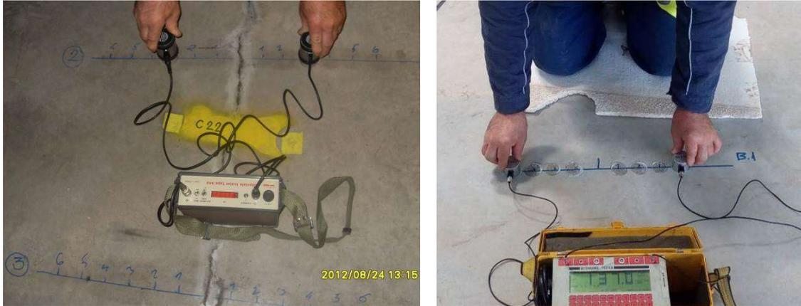
**Fig. 3.49 and 3.50 Ultrasonic diagnosis the depths of appeared cracks in Megapark Sofia (left) and in the industrial hybrid without expansion joints pavement of LIDL Kabile (right)**
