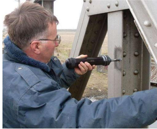
**Fig. 3.3 and 3.4. NDT of old metal bridge with a hardness testers of "Poldi" (left) and "HPS" (right)**
