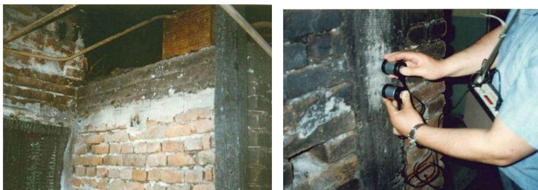
**Fig. 3:12 and 3:13. A look to part of the structure of the residential building at ul. Krum Popov after the fire in spring of 1997 and to one of sonic testing R/C column**
