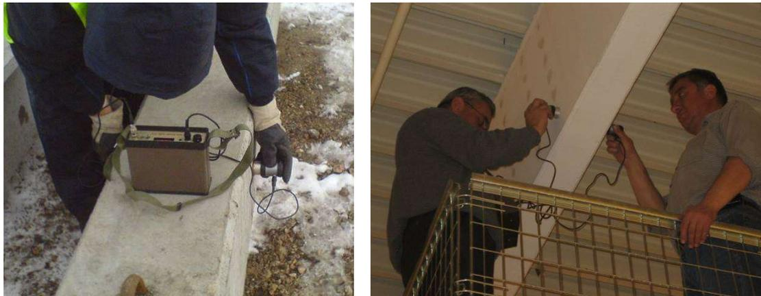
**Fig. 3.47 and 3.48 Ultrasonic testing for qualifying driving piles (left) and R/C girders of the prefabricated roof structures of BILLA hypermarkets (right)**
