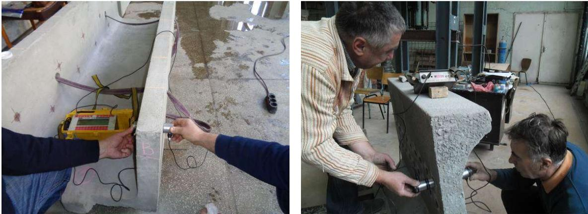
**Fig. 3.45 and 3.46 Ultrasonic sonic testing for the classification of precast ditches EKT 200/50 (left) and platform elements PEM 76 (right)**
