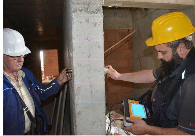
**Fig. 3.59 and 3.60 Ultrasonic diagnosis of cut drilling cores and monolithic wall with surface defects in an 8-storey building in Sofia (2018)**
