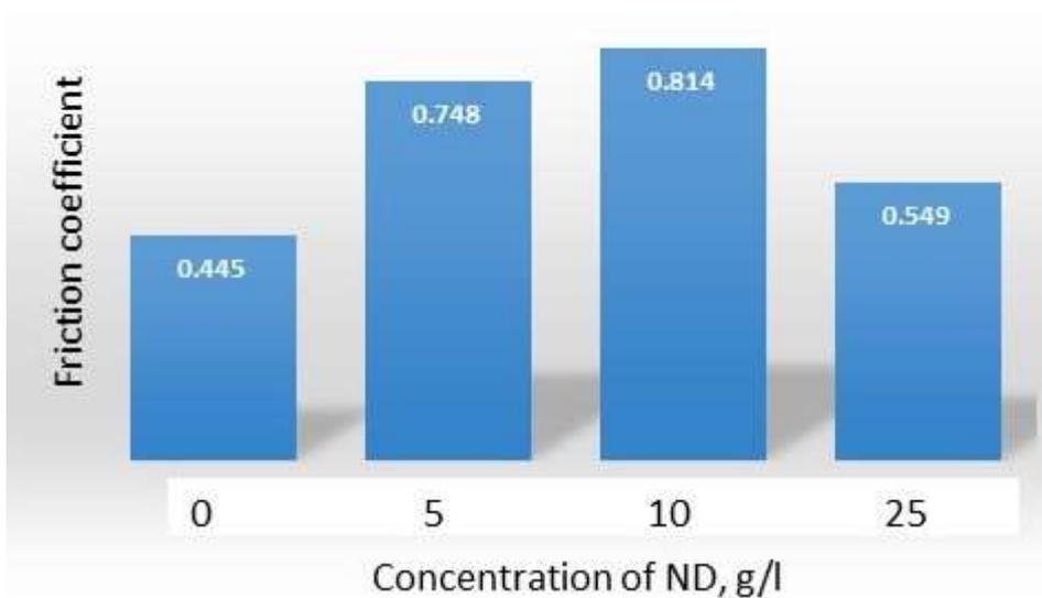
**Fig. 7. Friction coefficient of the composite coating at different concentrations of nanodiamonds**
