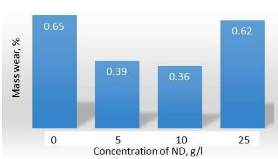
**Fig. 6. Wear resistance of the composite coating expressed as mass wear at different concentrations of nanodiamonds**
