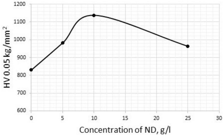
**Fig. 4. Microhardness of the composite coating at different concentrations of nanodiamonds**
