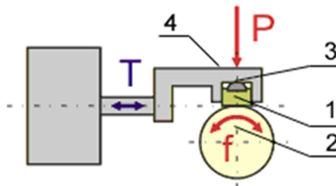
Fig. 1. Schematic view of a block-on-ring test unit
