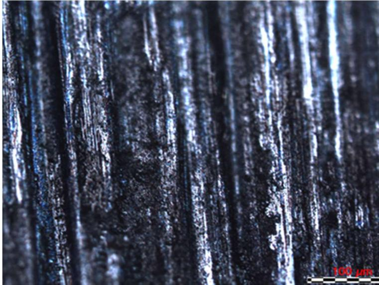
Fig. 10. Surface topography of sample with 25 g/l ND after the wear test. Applied load 165 N and sliding distance 500 m.
