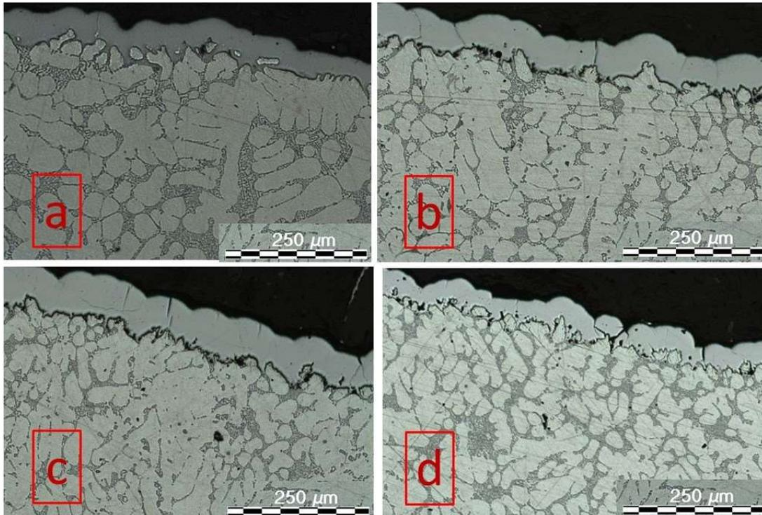
**Fig. 2. Micro images of coatings obtained from electrolytes with different  $C_{ND}$**
