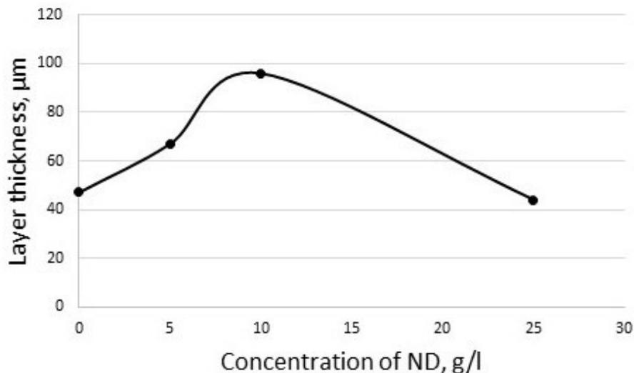
**Fig. 3. Coating thickness in relation with the  $C_{ND}$ , measured by microhardness tester**
