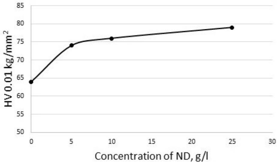
**Fig. 5. Microhardness of the aluminum matrix at different concentrations of nanodiamonds**
