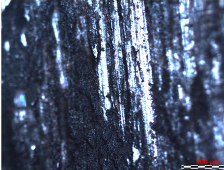
**Fig. 8.** Surface topography of sample with 5 g/l ND after the wear test. Applied load 165 N and sliding distance 500 m.
