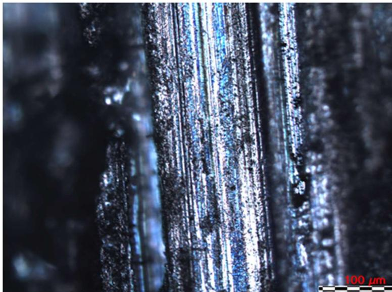
**Fig. 9.** Surface topography of sample with 10 g/l ND after the wear test. Applied load 165 N and sliding distance 500 m.
